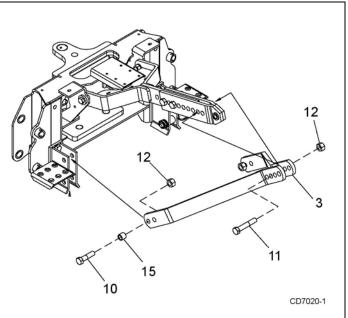
Figure 4. Offset Bar Installation
